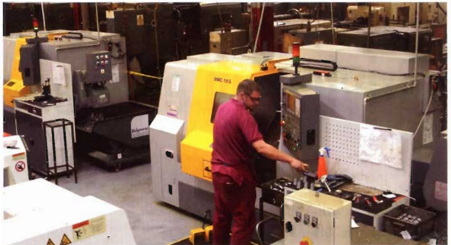
The DMC CNC lathes supplied by Leader CNC to LIC have demonstrated significant savings. Reduced changeover time plus higher speeds and feeds are put as the reasons for this performance
