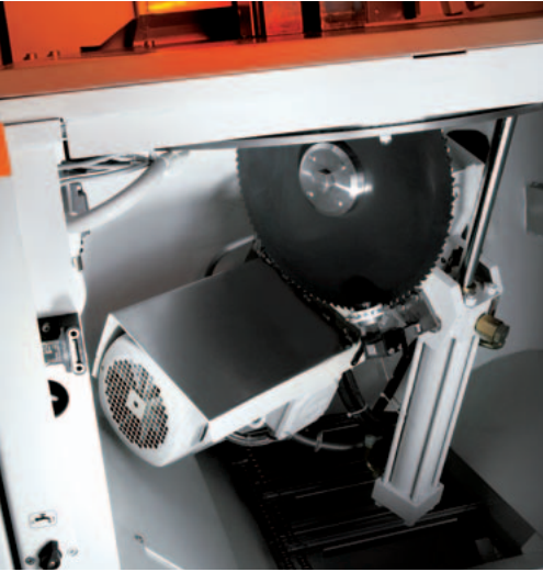
Generous access for easy saw blade change
