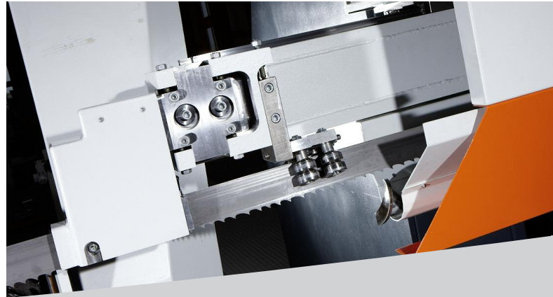
Rigid welding construction in horizontal position with pretensioned linear guides. Bandsaw blade guides with closed supply system. Integrated tool control sensors.
