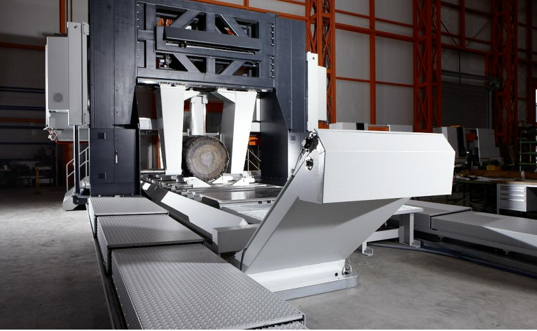
Chip conveyor with a conveying width of 1.250 mm (49.2") and an ejection height of 1.100 mm (43.3").
