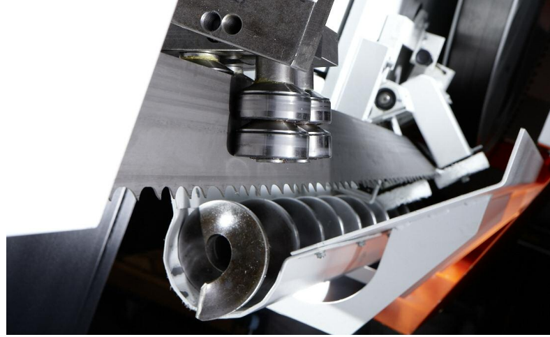
Screw conveyor in saw head with double chip brush.
